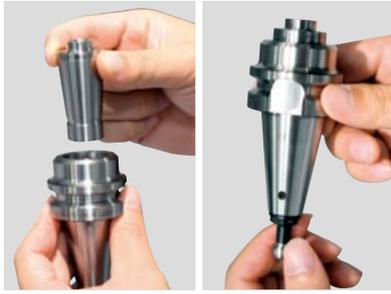
**① 仮締め (BT30) Initial Tightening**
